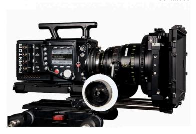
The Phantom Flex 4K is Vision Research's latest offering for the Motion Picture market. Lower image noise and a higher dynamic range than the Flex 2K make this a very attractive option for ultra high-speed digital capture. The Flex 4K has in camera controls for menu and trigger functions and offers 64GB of internal storage.
